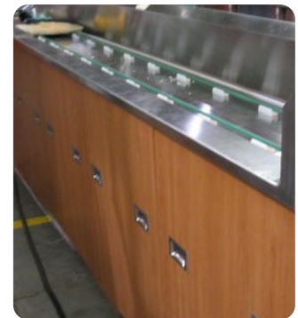
Polycord Conveyor Drop-Off
